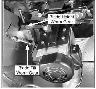
Figure 79. Gear lubrication.
